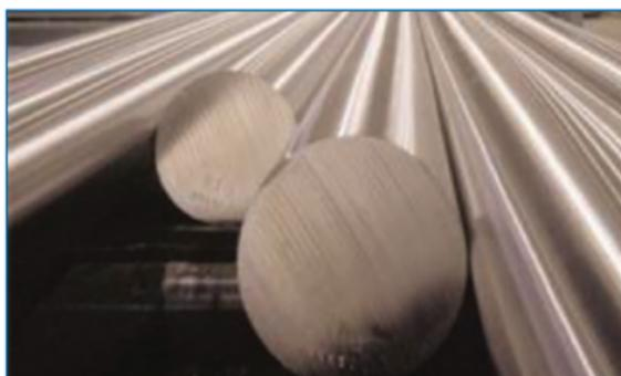
**FIGURE 3:** Titanium forged billets
