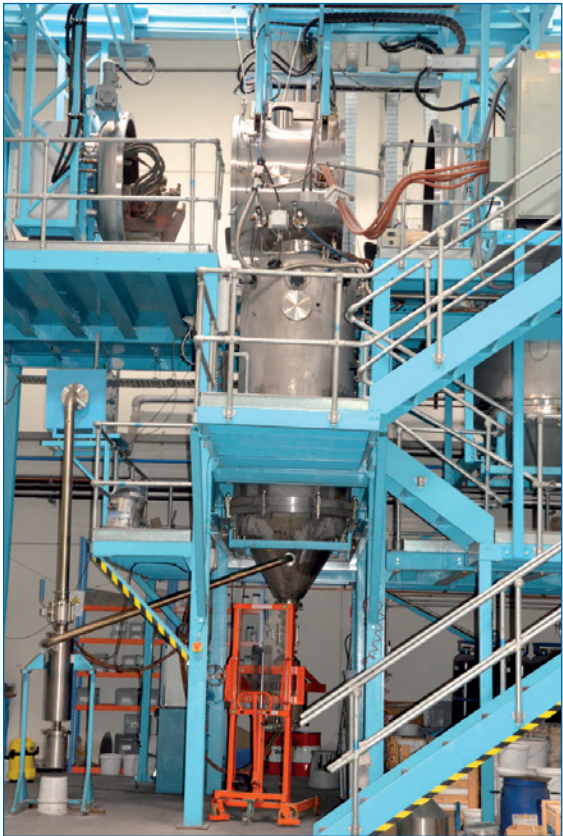
FIGURE 3: The VIM gas atomizer at Metallised in Irun, Spain
