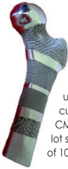
FIGURE 3: Demonstrator femur illustrating different porous scaffold designs
