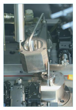
3. The cutter head is mounted into the thread whirling unit.
