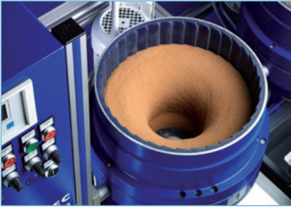
FIGURE 1: The right mixture for precision: disc finishing machine.
